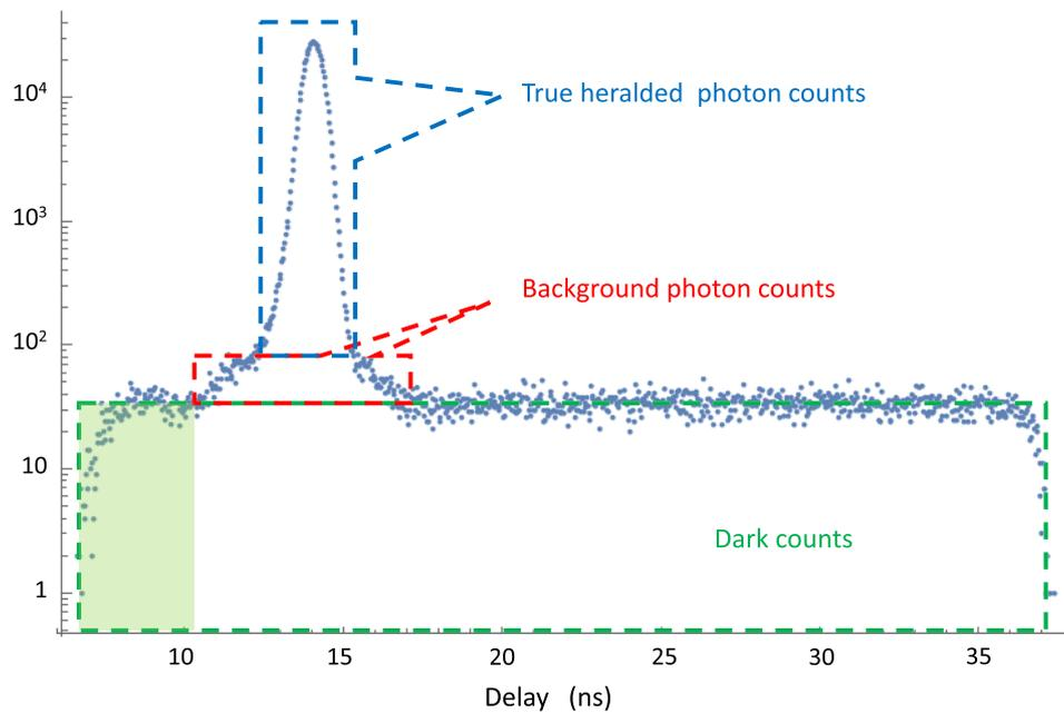
**Figure 2.** Histogram of the detections acquired in one run by one of the INRiM HBT gated SPADs, with a 30 ns detection window. The true heralded photons (Her), background photons (Bkg) and dark count (Dark) contributions can be clearly seen. The green shaded area indicates the dark counts forbidding the SPAD to detect a photon from the HSPS.
