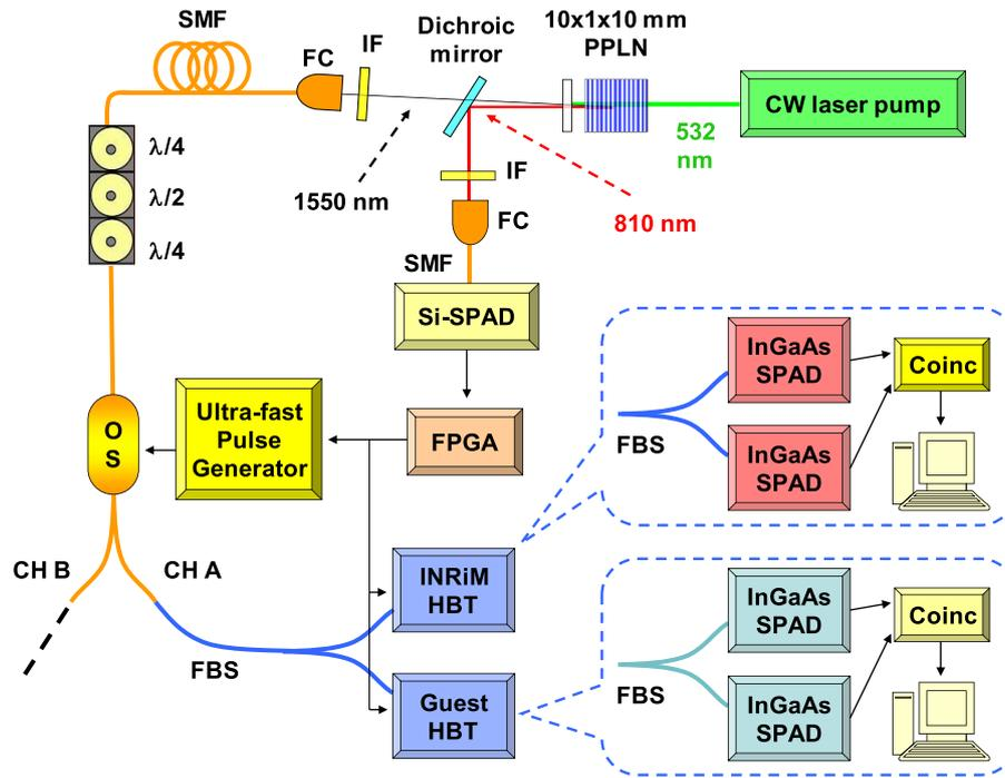
**Figure 1.** Experimental setup. PPLN: periodically-poled lithium niobate. FC: fiber coupler. SMF: single-mode fiber.  $\lambda/4$ : quarter-wave fiber paddle.  $\lambda/2$ : half-wave fiber paddle. OS: optical shutter. FPGA: field programmable gate array. FBS: fiber beam splitter. HBT: Hanbury-Brown & Twiss interferometer. Coinc: time-tagging coincidence electronics.
